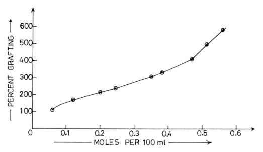
**Figure 3** Effect of molar concentration on the percentage of grafting of acrylamide on PVPy, (PVPy, 100 mg; water, 3 mL; temperature, 112–115°C; total dose, 2.4 MR).
