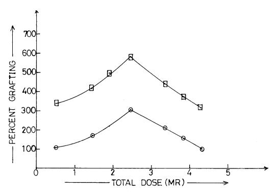
**Figure 1** Effect of total dose on the percentage of grafting of acrylamide on PVPy (PVPy, 100 mg; water, 3 mL; temperature, 112–115°C): (O—O) acrylamide, 0.014 mol; (O—O) acrylamide, 0.028 mol.
